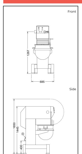
Electric 220-240/380-415 V/3 ph/50 Supply voltage: Electrical power, max: 1.54 kW **Total Watts:** 1.54 kW Capacity: ISO 9001; ISO 14001 kg/ Performance (up to): Cycle 60 litres Capacity: Key Information: External dimensions, 685 mm Width: External dimensions, 1087 mm Depth: External dimensions, Height: 1445 mm **Shipping weight:** 332 kg ISO 9001; ISO 14001 kg with Spiral hook **Cold water paste:**
